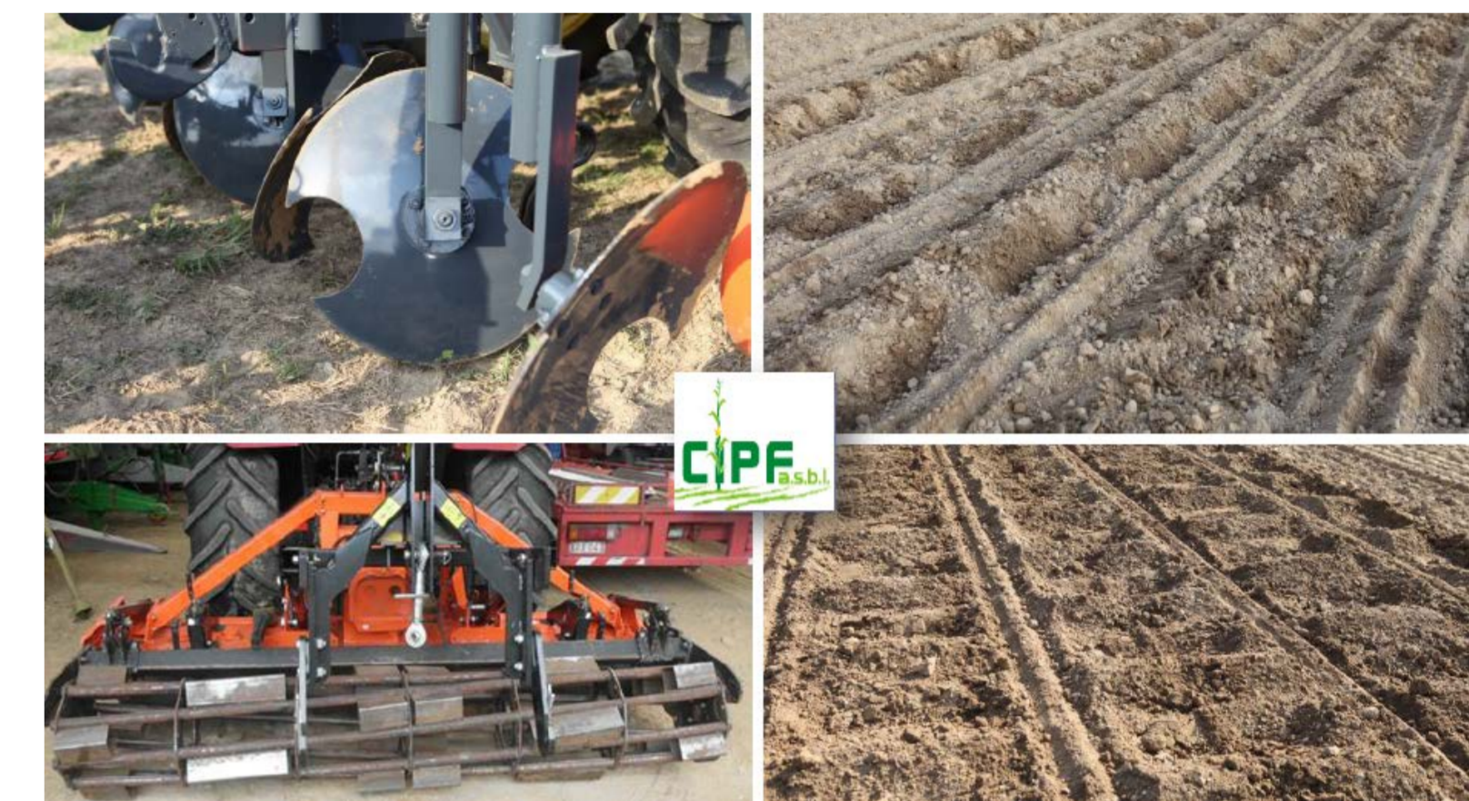
Figure 2: Erosion reduction with disc plough (above) or drum plough (below) 8 .
